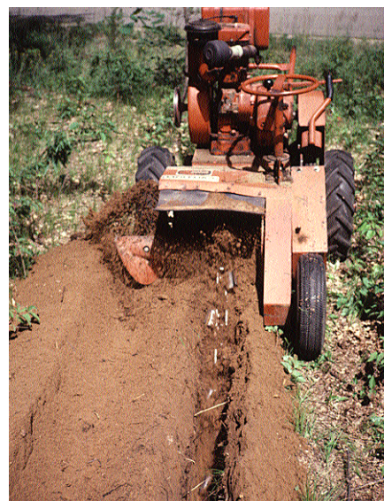
Example 3b. Oak wilt trenching.
